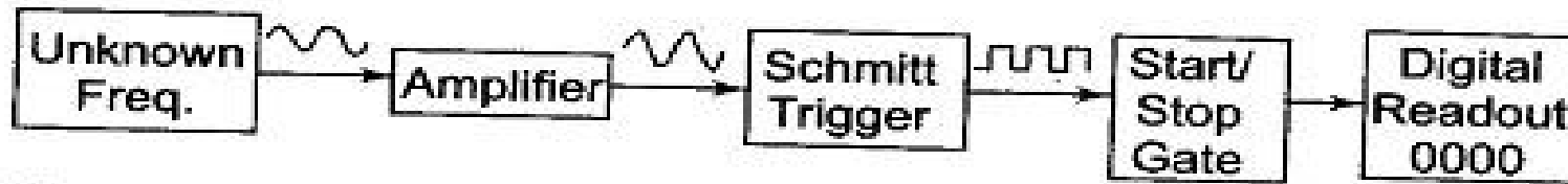
Fig. 6.5 Basic Circuit of a Digital Frequency Meter
